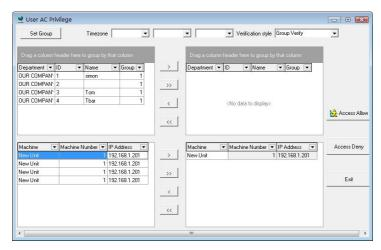
10 after users and equipment is selected, click on "allows" button, the group Time period which is used by user in the critical periods will be assigned to the selected devices. After distribution is successful, prompt will appear shown as following
