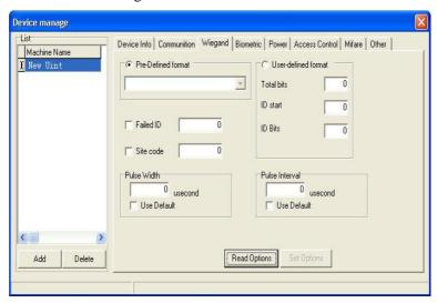
Click **Read Option** to obtain all kinds of wiegand parameter which store in the fingerprint machine; there are four **Defined Formats** in the drag –down volume to select. to choose a wiegand 26 or wiegand 34 is avaliable.
