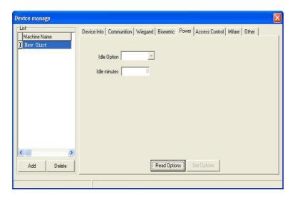
Firstly read the parameter of **Power Management**, modify the state of **Idle Setup** and minutes of **Idle Time**, then click the
